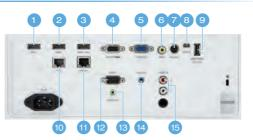
1.HDMI 1 2.HDMI 2 3.HDMI 3 / MHL 4.MONITOR OUT 5.CONPUTER IN 6.VIDEO 7.3D SYNC 8.SERVICE 9.USB POWER 10.RJ45 11.HDBaseT 12.RS-232C 13.AUDIO OUT 14.AUDIO IN 15.AUDIO IN (L/R)
